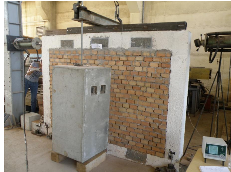
Fig.4 Solid bricks masonry infill wall
