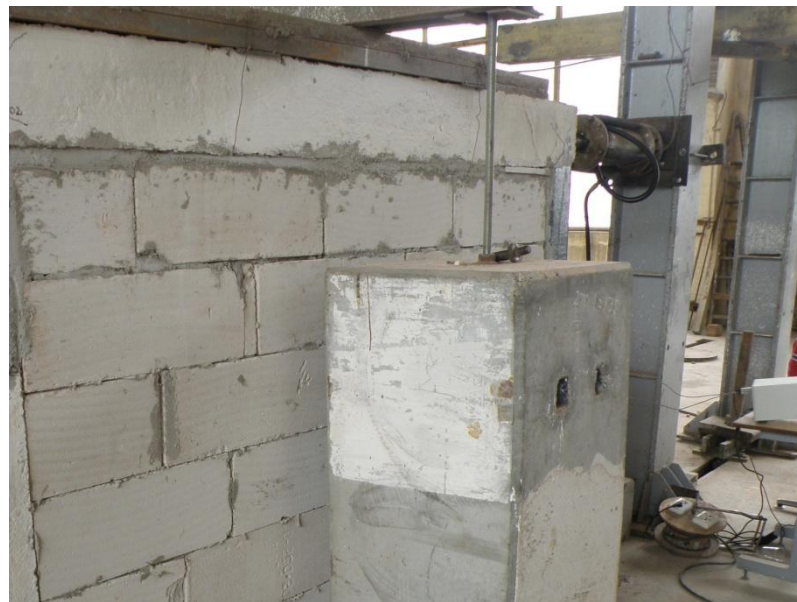
Fig.2 Cellular concrete masonry infill wall
